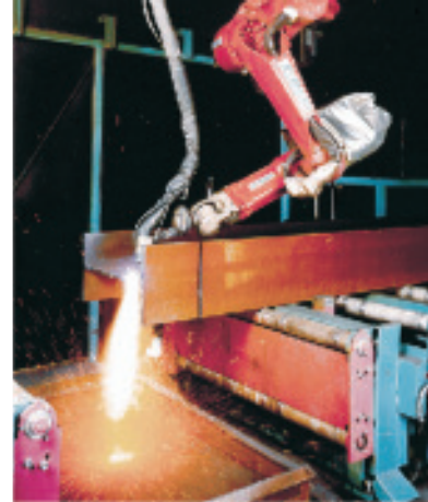
Plasma cutting with robot
